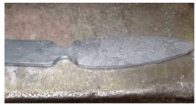
Using a spring fuller or a guillotine tool fuller the tree at about 3 inches. The one in the image is a bit long. It can be fixed by cutting or filing a new pointed end.
