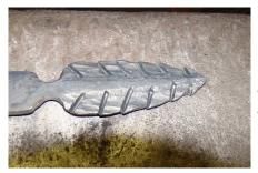
Then using a treadle hammer, a helper or a hold down hot cut the branches. You can leave them deep as illustrated or cut through it is a matter of personal preference.
