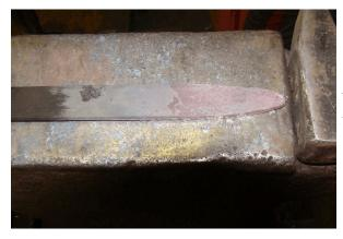
Using a bar of 3/16 x 1 inch taper the end. I do not bring it to too much of a point as I want to drill a hole at the top.
