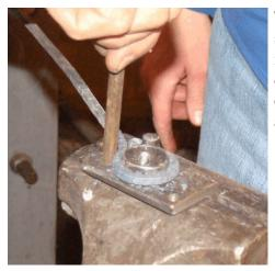
The jig is made around 1 inch OD pipe welded to an angle. A short stub is placed about 7 O'clock. Heat a little over 3 inches of your skewer. Catch the scroll behind the stub, pull outward as you wrap the skewer around the pipe. When you clear the second hole (about 5 O'clock) insert the taller stub and bend the skewer back on it.
