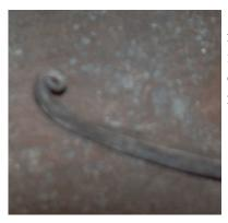
Start by cutting either 14 3/8 inch lengths of 3/16 square rod. (This equates to 10 pieces from a 12 foot length) or 15 inches of 3/16 round rod. Taper and scroll the end. Depending on your jig you may want to taper the square a bit more then the round to give you more room. See step 3.
